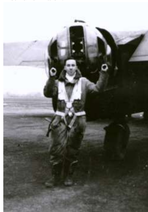
Photo of me (Mike Cassidy) holding guns at my tail turret in MK III Halifax 1944. The 4 guns are Browning 303 and fire 1,150 rounds each per minute and synchronized for 450 yards.
